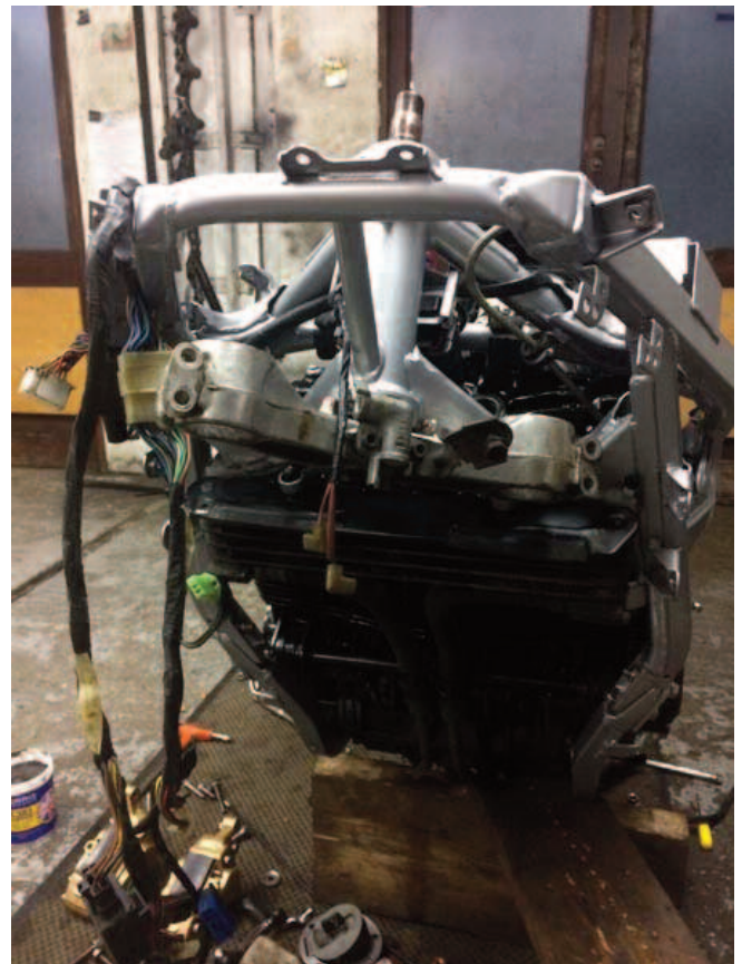
Front end removed so I could fit the bearings correctly. One step forward, one step back
