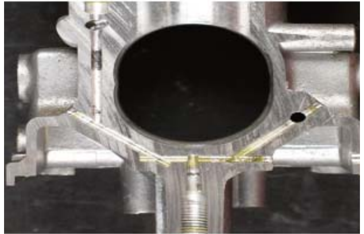
Figure 1 shows the cross section of the carb cut through the primary drillings. Tar can be seen as a golden colour deposit.
