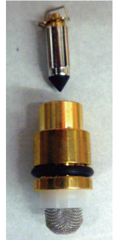
Float kit; main part is the needle and seat
