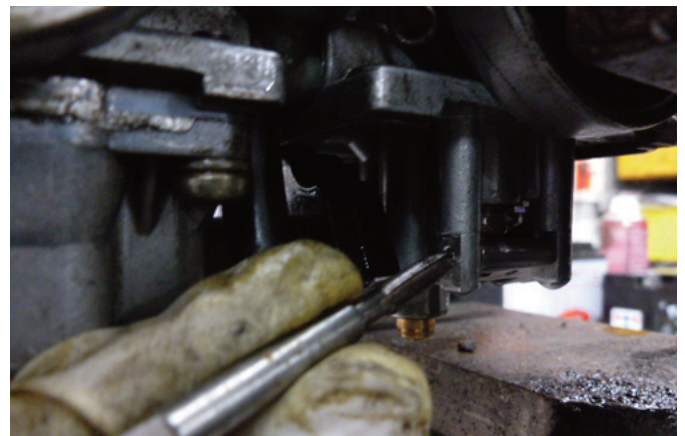
Tap out float pin carefully
