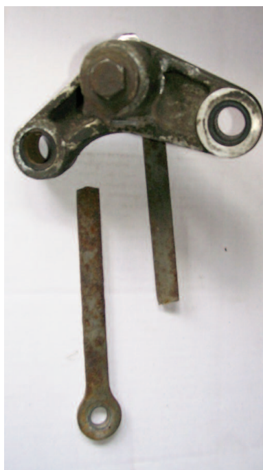
Snapped Suspension Linkage Arm caused by lack of proper servicing
