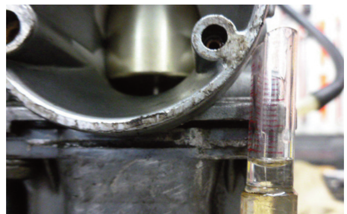
Fuel Level below gasket level
