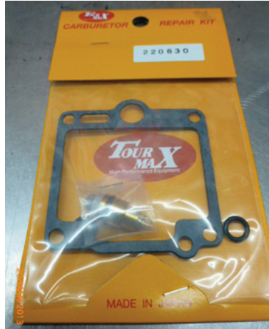
Float kit; main part is the needle and seat
